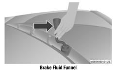
3. After topping up, remove the funnel with the extension pipe.
