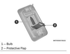
3. Close protective flap (2) and install roof light in its housing, making sure that it is locked in place.
