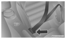
**Inserting Latch Plate Into Buckle**
