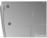
Inner Wheel Liner Fasteners
